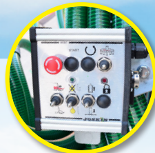
ELECTROHYDRAULIC CONTROL Automaton with control box in the cabin
