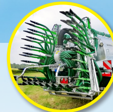
HYDRAULIC FOLDING SYSTEM • BASIC: single (3 parts) • START: double (5 parts)
